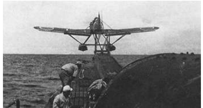
The aircraft carried two incendiary 168 pound bombs and a crew of two. The "Glen" was launched via catapult from a I-25 class Japanese submarine.
